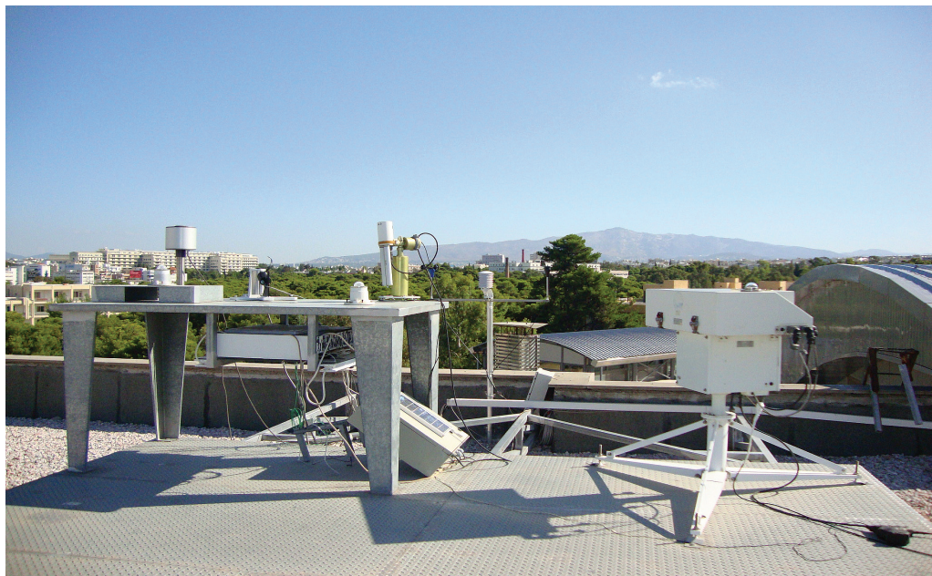
Fig. 13. The CEEH – BRFAA station for measuring the quality of the atmospheric environment, part of the global network for ozone/ultraviolet radiation measurements.
